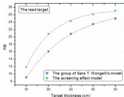
**Figure 7.** A comparison of neutron multiplicity ( $n/p$ ) per incident proton calculated by the research group of Sara T. Mongelli et al. and by the screening effect model
