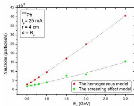
**Figure 6.** A comparison of the number of neutrons emitted from spallation reaction calculated with  $^{206}\text{Pb}$  bombarded with proton energies from 0.5 GeV to 3.0 GeV in the screening effect model and the homogeneous model
