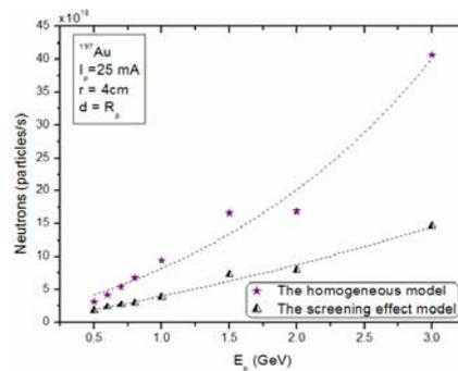
**Figure 10.** A comparison of the number of neutrons emitted from spallation reaction calculated with  $^{197}\text{Au}$  bombarded with proton energies from 0.5 GeV to 3.0 GeV in the screening effect model and the homogeneous model
