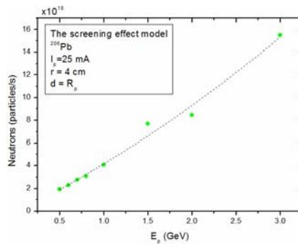
**Figure 5.** The number of neutrons emitted from spallation reaction calculated with  $^{206}\text{Pb}$  bombarded with proton energies from 0.5 GeV to 3.0 GeV in the screening effect model
