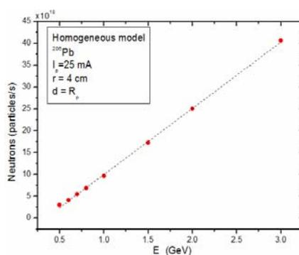
**Figure 1.** The number of neutrons emitted from spallation reaction calculated with  $^{204}\text{Pb}$  bombarded with proton energies from 0.5 GeV to 3.0 GeV in homogeneous model
