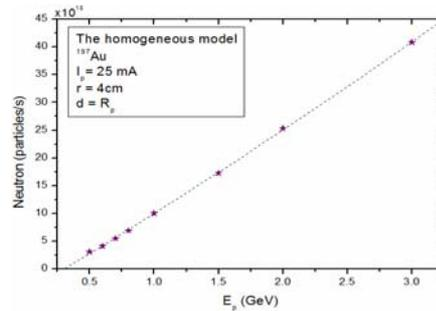
**Figure 4.** The number of neutrons emitted from spallation reaction calculated with  $^{197}\text{Au}$  in range of proton energies from 0.5 GeV to 3.0 GeV
