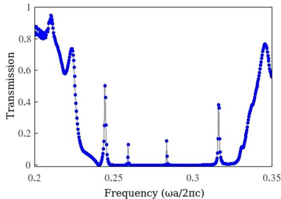
**Figure 4.** Transmission spectrum of photonic crystal L3 nanocavity. A wide band gap can be seen in transmission spectrum. The gap extends from  $u = 0.245$  to  $u = 0.32$ .
