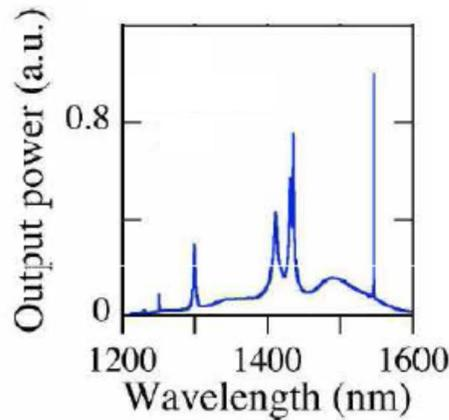
**Figure 5.** Photoluminescence spectrum of photonic crystal L3 nanocavity
