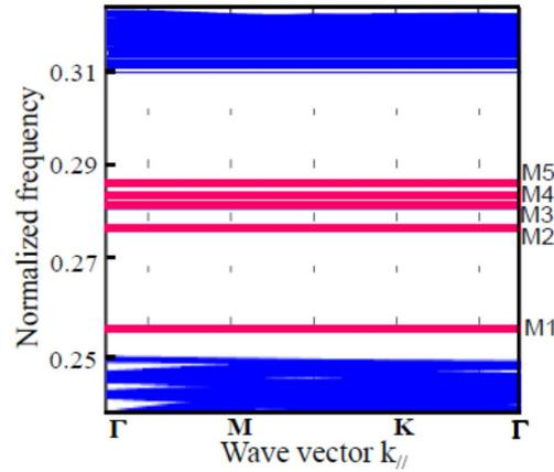
**Figure 2.** Calculated dispersion diagram of a silicon photonic crystal L3 nanocavity. The white area corresponds to the photonic band gap. The defect modes of the L3 nanocavity which appear as horizontal pink solid lines in the gap, are numbered from M1 to M5.
