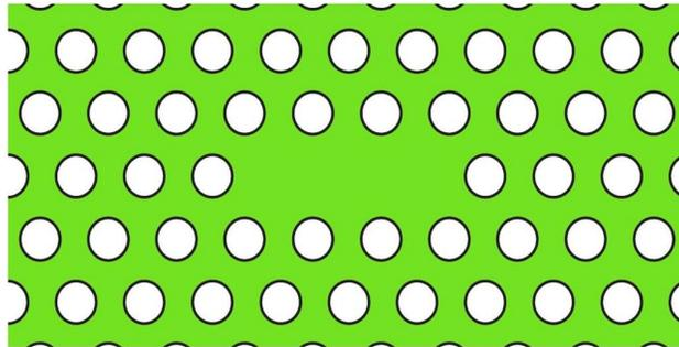
**Figure 1.** A schematic representation of the 2D photonic crystal L3 nanocavity which is based on a three-missing-point defect in a triangular lattice. The lattice constant is  $a$  and the hole radius is  $r = 0.3a$ .
