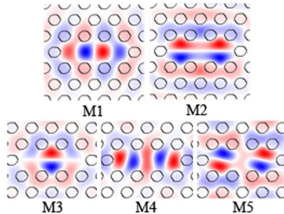
**Figure 3.** The diagram shows the magnetic field distribution of resonant modes of L3 nanocavity, numbered from M1 to M5.
